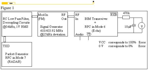
(S+N)/N was measured by taking the ratio of the Audio output level with & without FM deviation.
